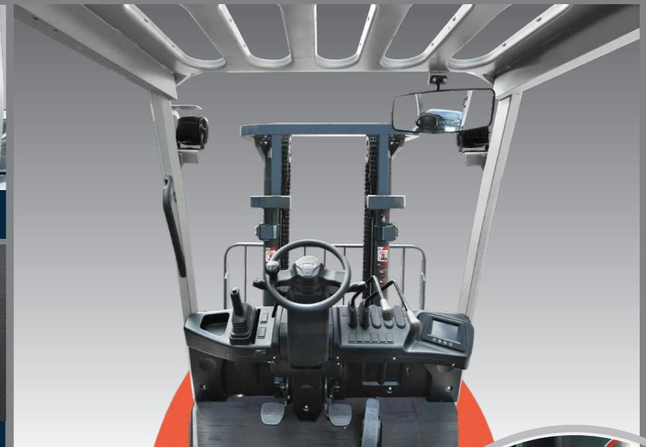
Wide view mast optimizes the blind area of operation vision and ensures comfortable and safe operation;
