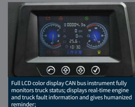
Full LCD color display CAN bus instrument fully monitors truck status; displays real-time engine and truck fault information and gives humanized reminder;
