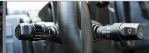
The standard configuration of electro-hydraulic reversing and steering handle and lamp combination handle improves the operation convenience;
