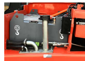
The hydraulic oil tank is located on the left side for easy filling and checking.
