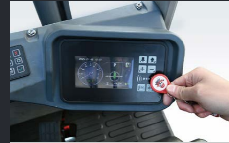
The integrated card swiping function of the instrument meets the requirements of TSG 81.
