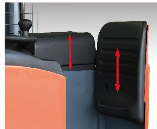
Adjustable backrest and armrest help reduce fatigue
