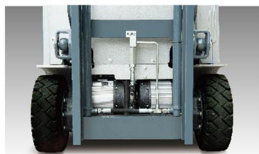
Front wheel dual drive motors provide more power.
