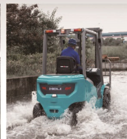
After 10mins wading test, the vehicle has no failure. (Water depth 200mm)
