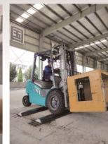
The truck passed simulation experiment of bumpy road.
