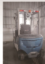
IP64 waterproof: the vehicle is powered on to simulate a 30mins test time at 500L atmosphere test, and the vehicle can continue to run without failures.
